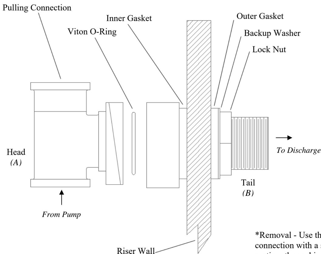
\*Removal - Use the pulling connection with a slight rocking motion, the rocking motion helps unseat the taper.
